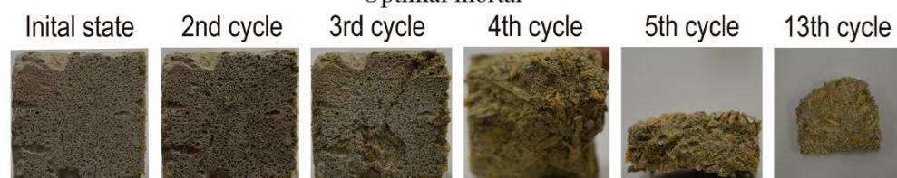
Optimal mortar with fibers
