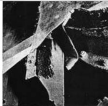
6. CLOSE-UP OF SKIN AT BOTTOM FRONT CORNER OF ESCAPE HATCH FIG. 15. FAILURE OF FRONT FUSELAGE AT 184 (3/4) 3 (327 TOTAL FLIGHTS)—G-ALYU.
