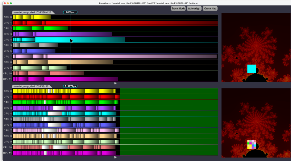
Figure 13: Comparing two traces with “tracking mode” enabled. When selecting a coarse grain task in one trace, the corresponding fine grain tasks are highlighted (in white color) in the other trace, and the accumulated execution time is indicated.
