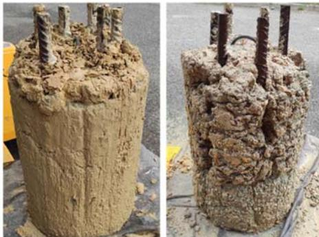
Figure 29: Experimental result for bad concrete & fresh slurry before (left) and after (right) cleaning
