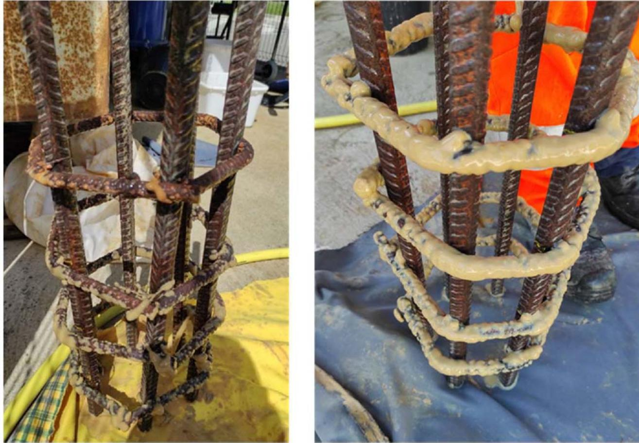
*Figure 17: Slurry deposits on rebars without exfiltration (left), with exfiltration (right)*
