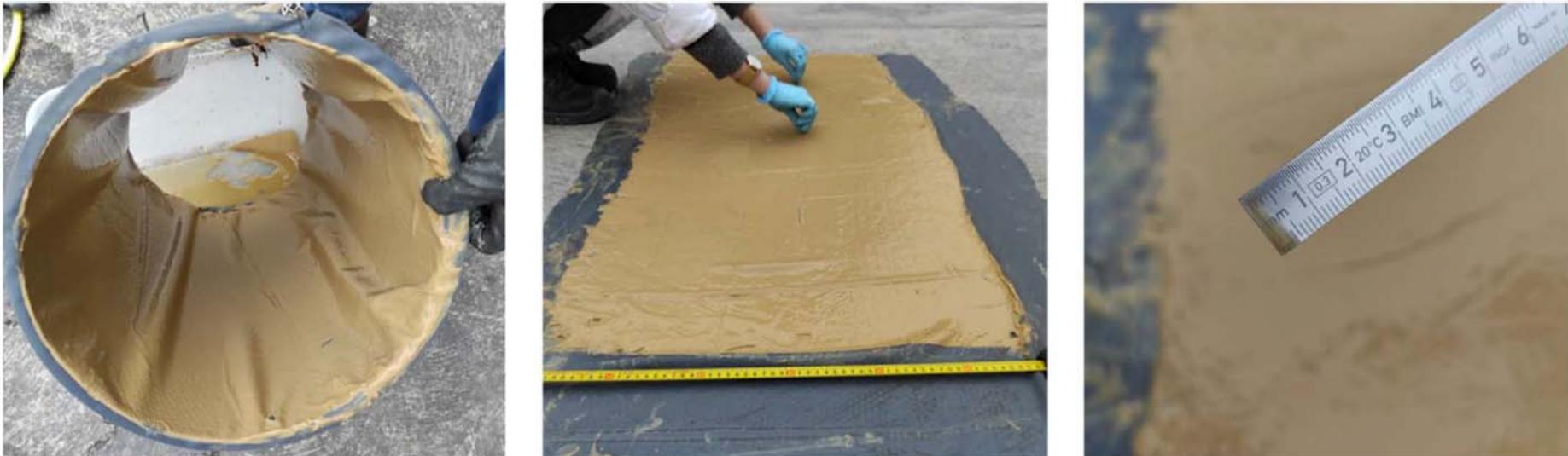
*Figure 11: Filter Cake formation at the interface of the geotextile*
