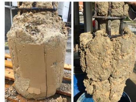
Figure 30: Experimental result for bad concrete & polluted slurry before (left) and after (right) cleaning
