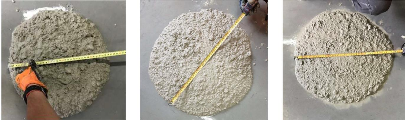
*Figure 23: Concrete spread diameters equal to 365 mm (left), 465 mm (center), and 560 mm (right)*
