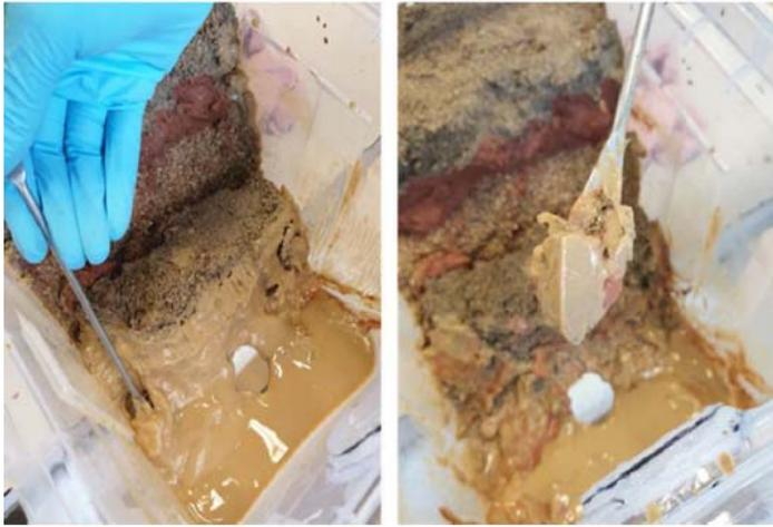
Figure 9: Resulting filter cake at interface of mixed soil
