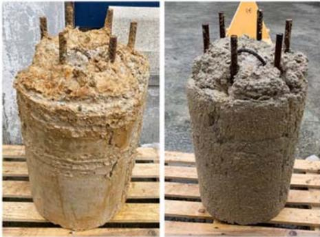
Figure 27: Experimental result for good concrete & fresh slurry before (left) and after (right) cleaning
