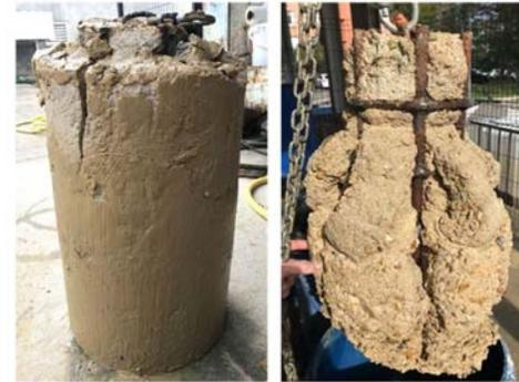
Figure 28: Experimental result for good concrete & polluted slurry before (left) and after (right) cleaning
