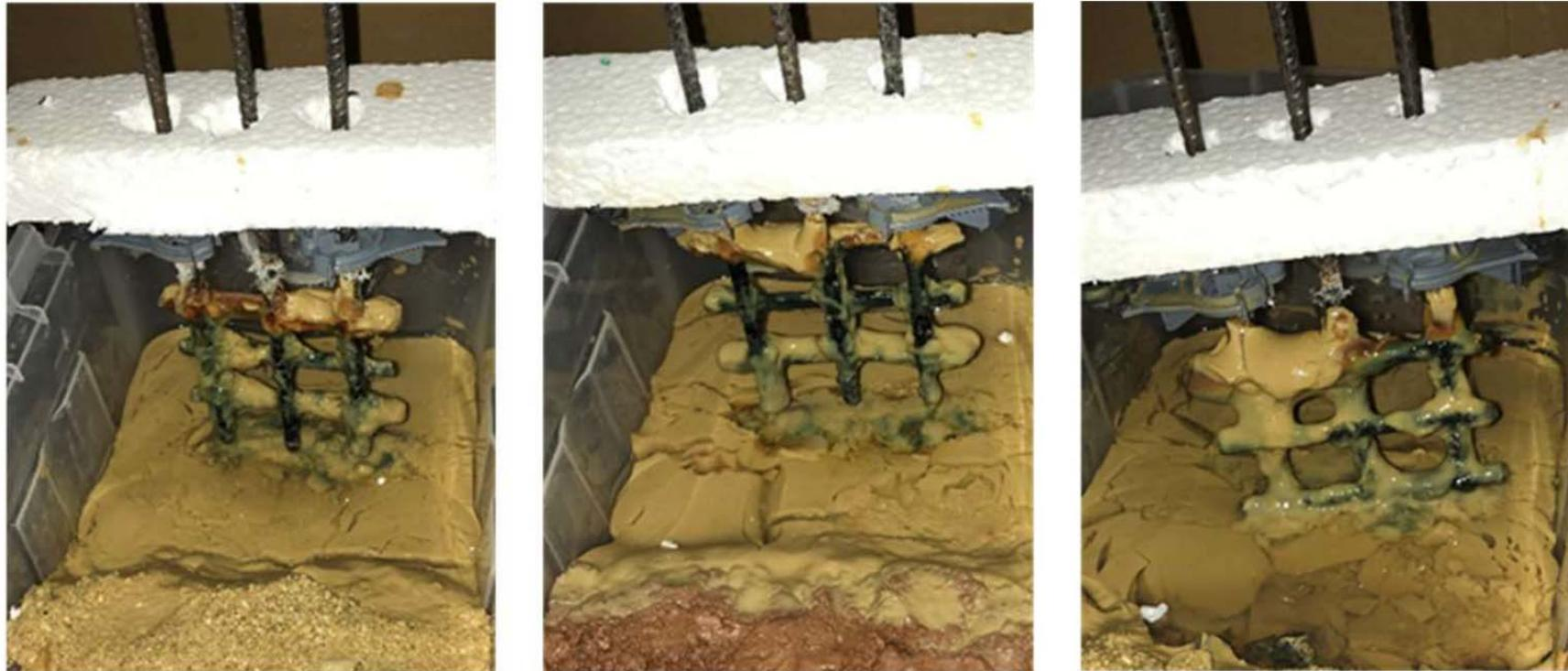
*Figure 11: Bentonite build up on the horizontal rebars*
