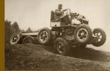
All-terrain car: The all-terrain car can descend slopes up to 65 degrees. England, 1926.
