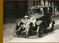
Car with shield for pedestrians: Invented for the purpose of reducing the number of accidents among pedestrians. Paris, 1924.
