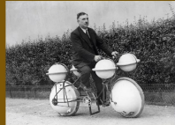
Amphibious bicycle: The land-and-water bike can carry a load of 1.8 tonnes. Paris, 1912.
