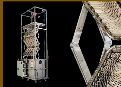
Mechanical tree , by Klaus Lackner, Professor in the School of Sustainable Engineering at Arizona State University. It shows that machines can be built to directly capture Carbon from the atmosphere.
