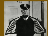
Electrically heated jacket: Electrically heated vest, developed for the traffic police in the United States, 1953. The power is supplied by electric contacts in the armpits.
