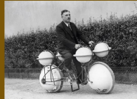
Airshipless bicycle: The land-and-water bike can carry a load of 1.8 tonnes. Paris, 1912.
