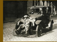
Car with shelter for pedestrians: Invented for the purpose of reducing the number of accidents among pedestrians. Paris, 1924.
