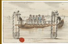
Manual dredger: Workers operated the so-called bucket dredger with their arms. Paris, 1912.
