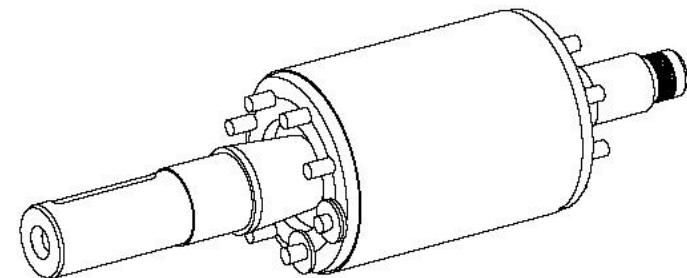
**[Short-cut necessary at the rotor to generate induced currents](#)**
