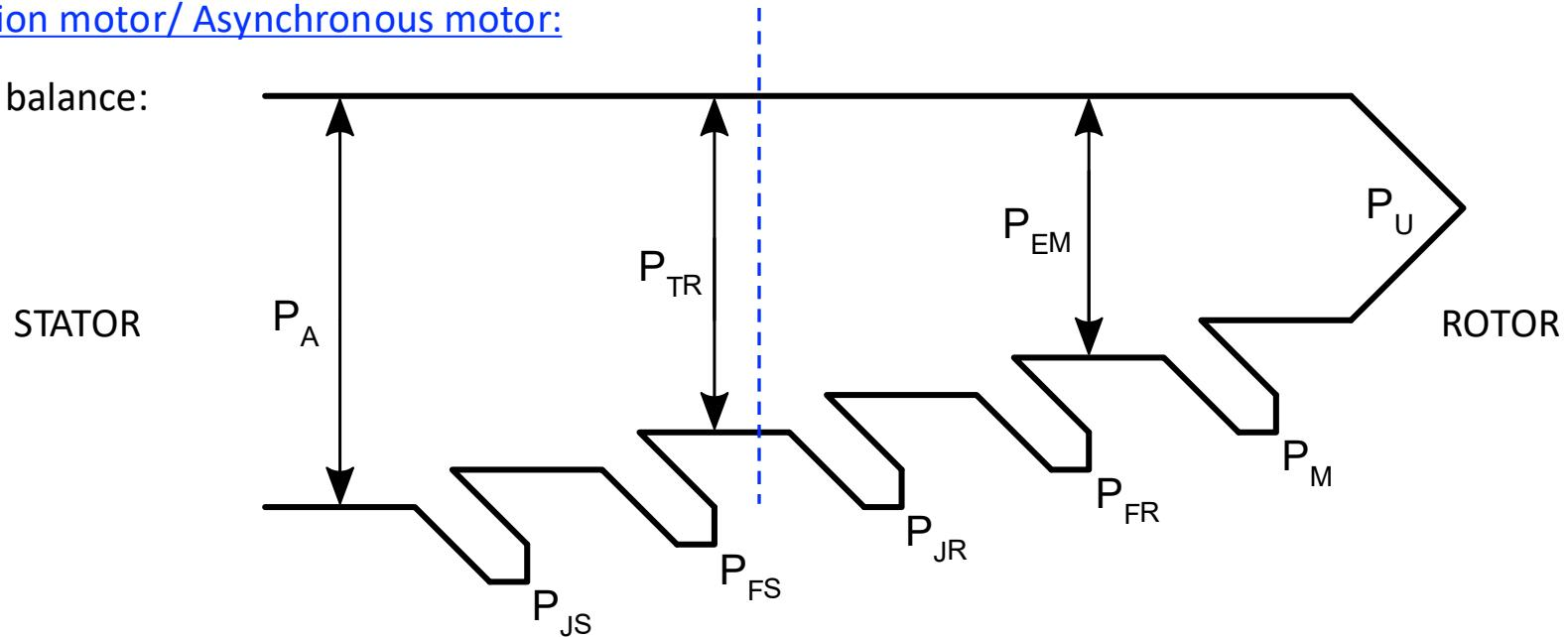
$P_a$ : Active power absorbed at the stator
