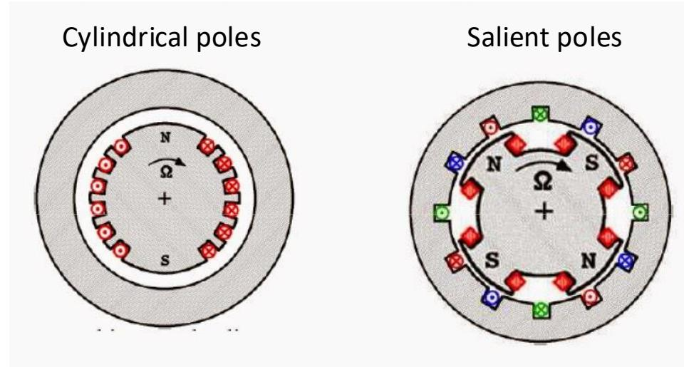
**Synchronous machine: The rotor rotates at the same speed as that of the rotation magnetic field**
