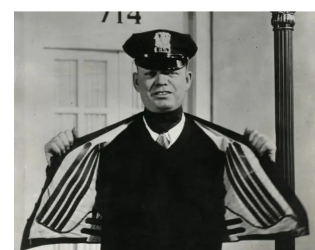
Electrically heated jacket: developed for the traffic police in the United States, 1932. The power is supplied by electric contacts in the street.
