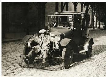
Car with shovel for pedestrians: Invented for the purpose of 'reducing the number of casualties among pedestrians;' Paris, 1924
