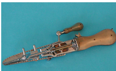
An early chainsaw, known as Osteotome, from 1780. The chainsaw as we know it appears to have begun life as a medical instrument—one used to assist in childbirth.
