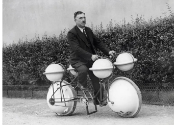
Amphibious bicycle: This land-and-water bike can carry a load of 120 pounds; Paris, 1932
