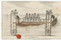
Manual dredger: Workers operated the so-called bucket dredger with their arms and legs using stepper boards.
