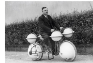
Amphibious bicycle: This land-and-water bike can carry a load of 120 pounds; Paris, 1932.
