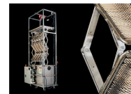
Mechanical tree, by Klaus Lackner, Professor in the School of Sustainable Engineering at Arizona State University. It shows that machines can be built to directly capture Carbon...
